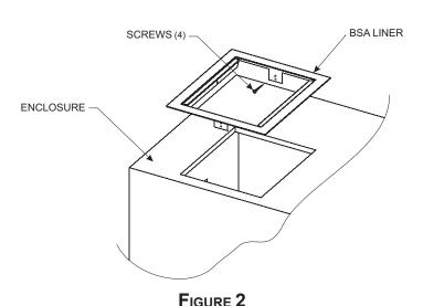
Attach one end of the Side Burner Hose to your Broilmaster® DPASBC Side Burner. The remaining end of the hose should be routed down through the bottom of the BSA Liner. Place the side burner into the BSA Liner and slide it completely to the rear of the
